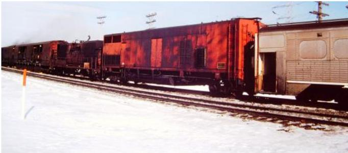
sual tank car which carries diesel fuel and (on RMS-5) 20,000 gallons of water, with an elevated fire fighting station and water nozzle because in warmer weather the right of way ahead of the
