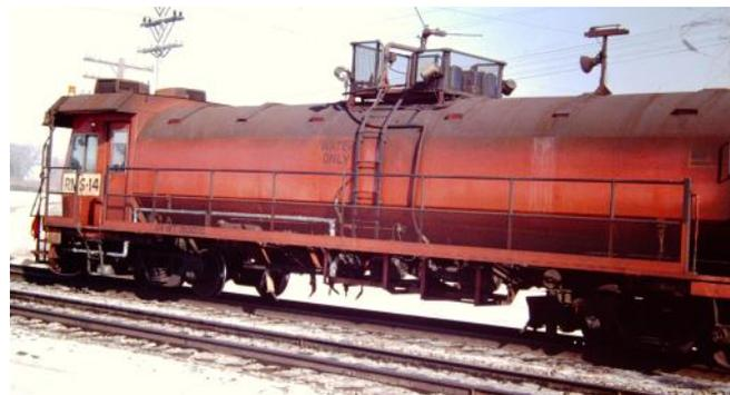
had at the end of the train a "B unit" locomotive without cab, actually a rebuilt F40PH-2M that Pandrol Jackson bought new.
