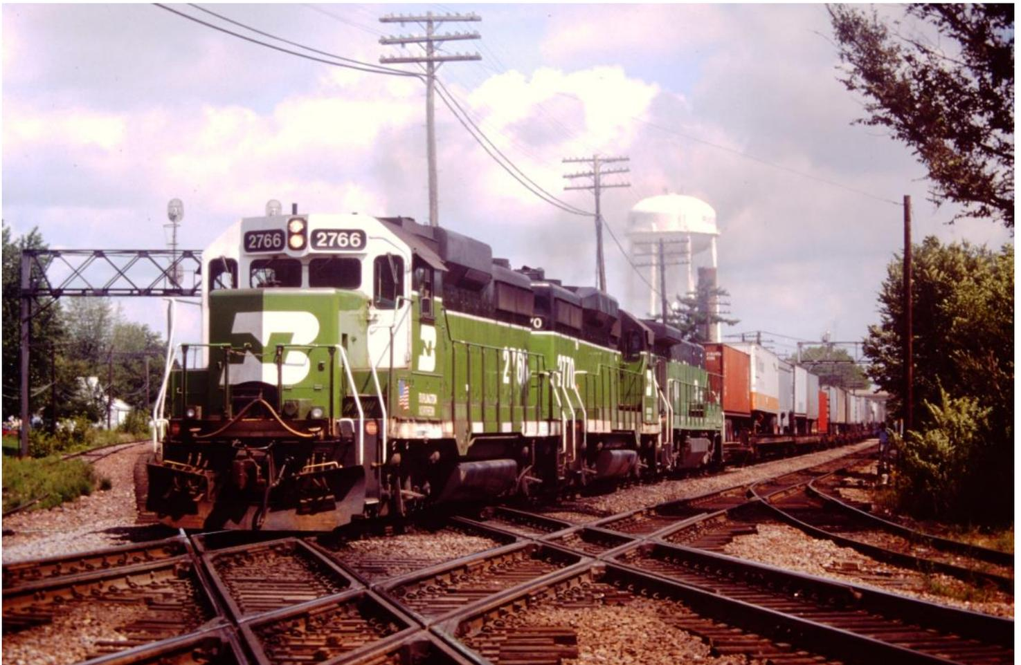
BN #2766 GP39E, rebuilt GP30 leads a piggyback train across the diamonds at Rochelle, IL. The photo was taken August 20, 1994. This would have been before the Union Pacific acquired the C&NW. It was also several years before the Rochelle Railfan Shelter was built. Photo by Dave Nelson
